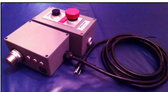
The 110V power connection ready to be installed on the telescope, as I mentioned in last month's report. It has a drive key switch, an emergency stop button, and a circuit breaker, as well as a power cord and 3 indicator lamps.
